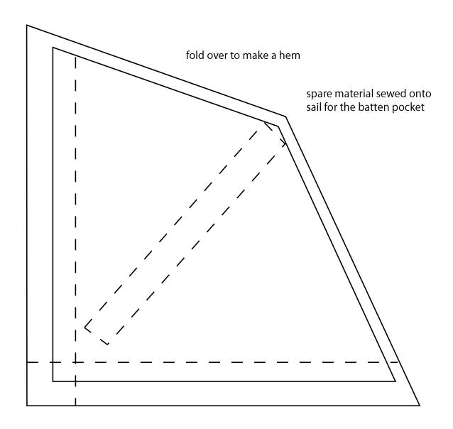
This corner folded to line to form a pocket for the mast Fold and sew to form a pocket for the boom.
