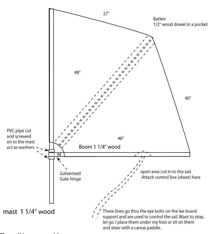
The sail is sewen with three pockets, one for the batten one for the mast and one for the boom
