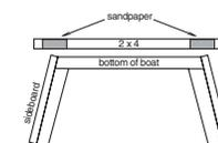
To attach bottom, turn boat upside-down, position bottom and tack each end and center as shown.
