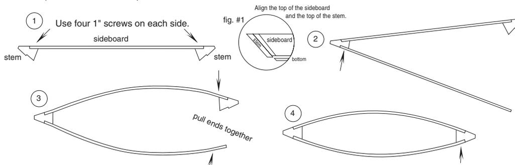
**No. 5 ATTACH THE RIBS TO THE SIDEBOARDS.** Attach rib #2 in center of hull (fig. #3) aligning sideboards as shown (fig. #2), glue and fasten with 1" screws. Install ribs #1 & #3, as shown (fig. #3). Rib #1 is beveled forward, rib #3 is beveled aft. Glue and fasten. When all ribs are attached, bevel bottom of sideboards as shown (fig. #4). See *E-Z TRICKS*.
